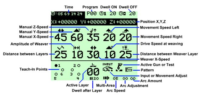
All standard functions for surfacing with remote control *RD2000* are available and optimized for manganese welding and hard facing.
